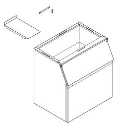
h. Seal the edges of the ice machine to the filler plate with the RTV sealant.
