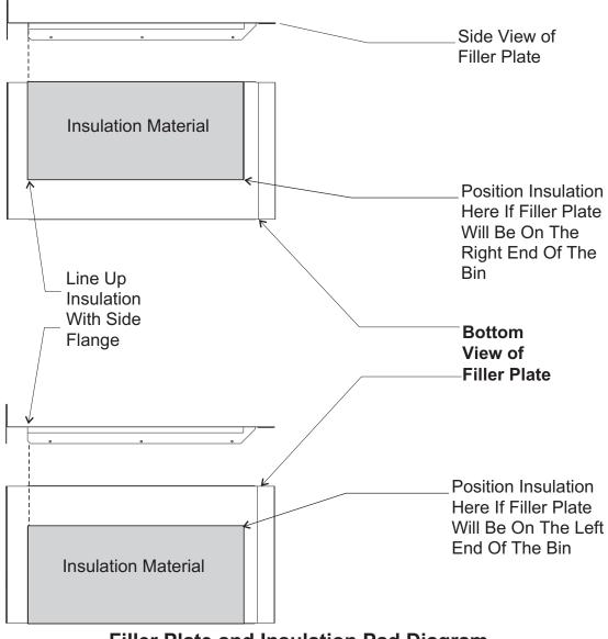
Filler Plate and Insulation Pad Diagram
